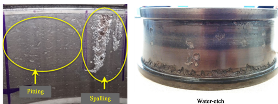
Fig. 2 Example of a localized defect (left) and distributed defect (right)
