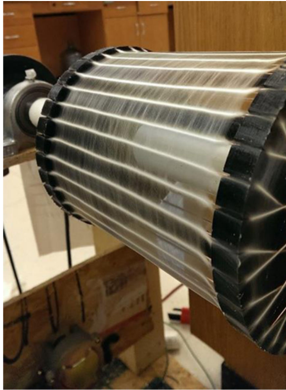
Figure 13. Rotating mandrel set-up for the electrospinning of aligned nanofibers showing the as-spun amorphous fibers aligned across the parallel copper wires on the rotating mandrel. Reproduced with permission. [156] Copyright 2016, The American Ceramic Society.
