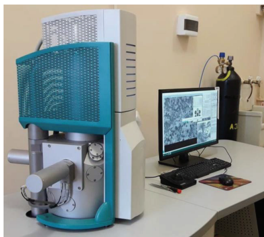
Fig. 1. Scanning electron microscope for microscopy of biofilms
