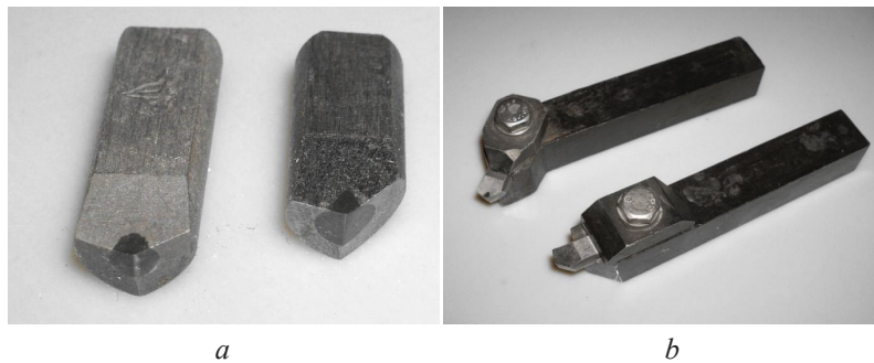
Fig. 1. Turning cutters with cutting material made of superhard materials: a – interchangeable tips; b – cutter assembly
