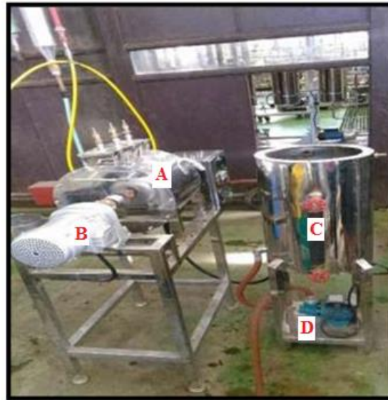
Figure 1. Saccharification Reactor used in the upscale enzymatic hydrolysis of pretreated banana pseudostem. The major components are reaction tank with rotating screw and jacket (A), motor (B), electrically-heated water drum for temperature control (C) and water pump (D).
