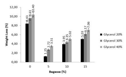
Figure 8. Biodegradation Test Value of Biodegradable Plastics
