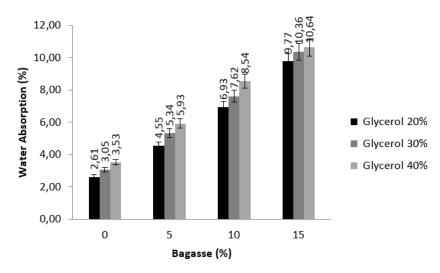
Figure 3. Biodegradable Plastic Water Absorption Value
