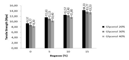
Figure 5. Biodegradable Plastic Tensile Strength Test Value
