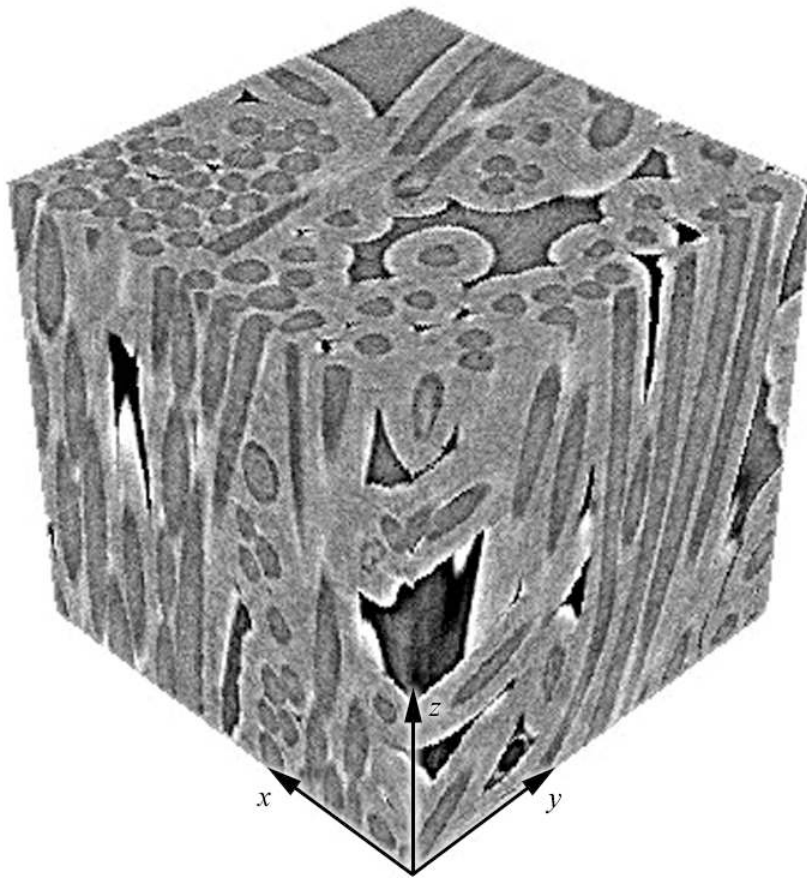
Figure 2.27. A synchrotron microtomography of a 3.3 \text{ mm}^2 (side length < 1.5 \text{ mm} ) cubic sample of a C/C composite. Voxel size is 7.45 \mu\text{m} .
