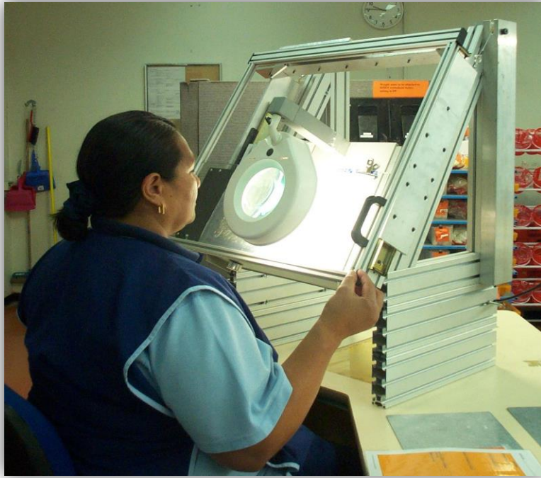
Figure 4.16: The Modified Dark Fibre Detector for AWTA Benzyl Test Method (Australian Wool Innovation Project, 2005)
