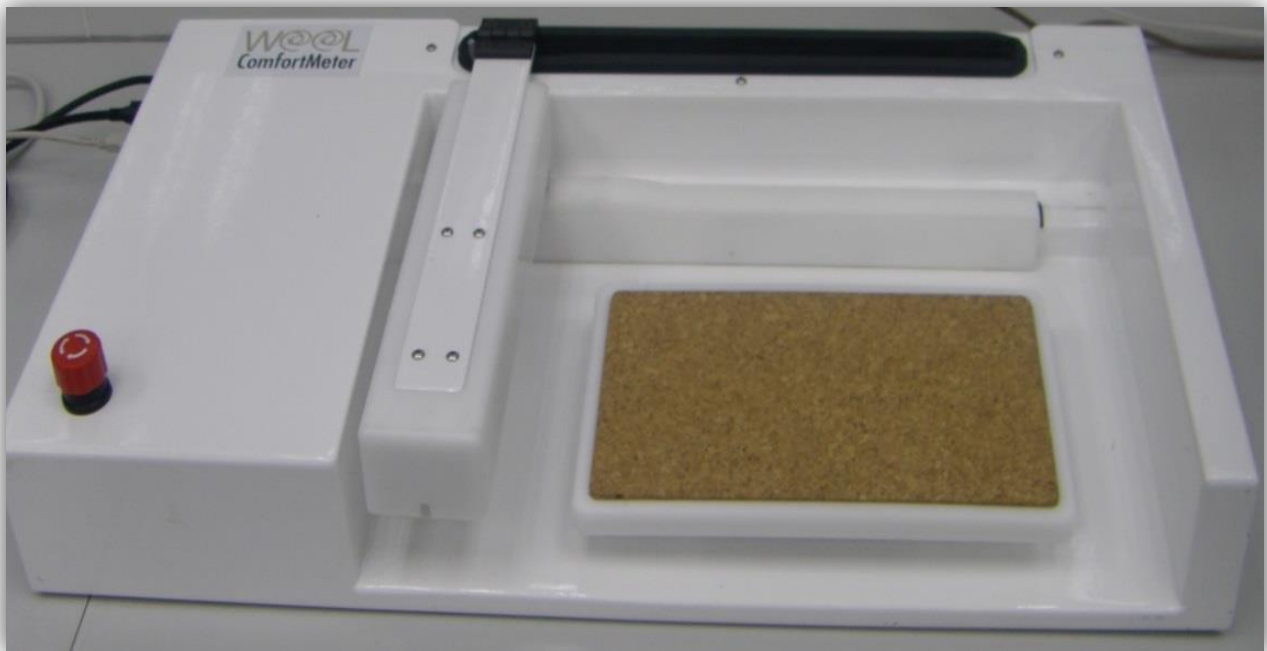
Figure 5.11: The Wool ComfortMeter (Sheep CRC, 2013)
