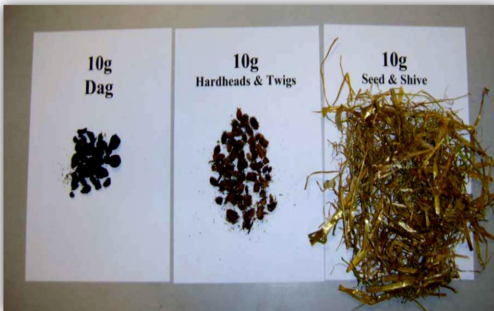
Figure 3.6: Different Types of Vegetable matter found in wool (Wool Testing Authority Europe, 2014).
