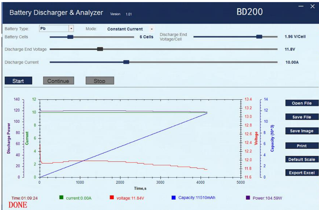
Fig. 3 Battery discharger software screenshot showing the discharge settings.
