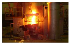
Fig. 6 Teaming of liquid melt into the oneton ladle.
