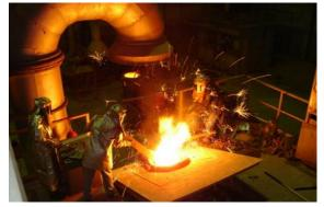
**Fig. 5** De-slagging process at the one-ton induction furnace.
