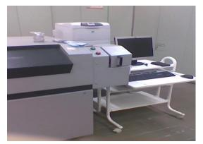
**Fig. 4** Spectro analytical instrument used for the determination of the chemical compositions of ferrous and non-ferrous metals.
