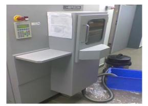
Fig. 3 Spectro analytical instrument used to polish cast or rolled material prior to the determination of the chemical compositions.
