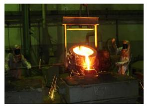
Fig. 7 Casting of roof hangers.
