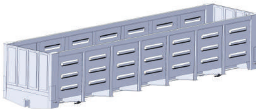
Fig. 1.11 Bearing structure of a gondola wagon model 12-757
