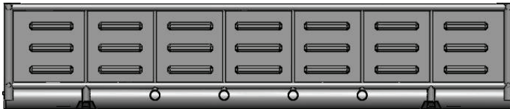
Fig. 1.13 Optimized bearing structure of gondola wagon model 12-757 (side view)
