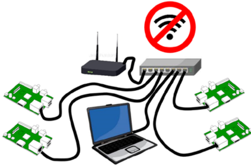
Figure 15. Networking Configuration with an Internal Ethernet Connection.
