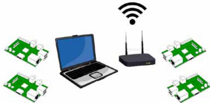
Figure 13. Networking Configuration with WLAN Through a COTS Router.
