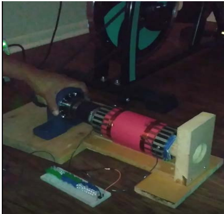
Figure 56. 120 LEDs connected to TENG with Stationary Bike
