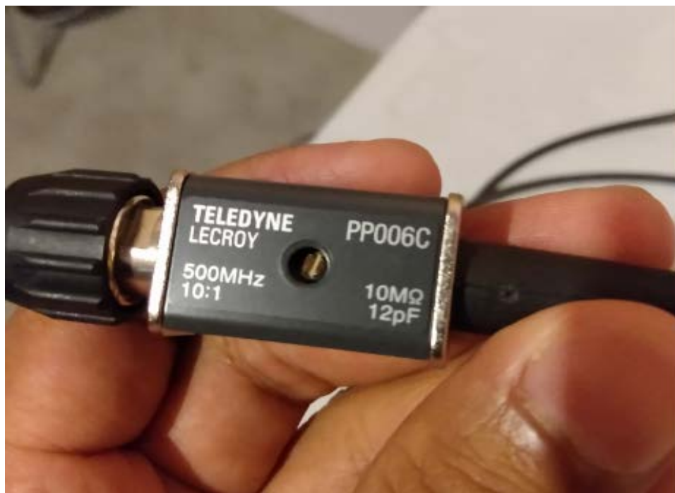
Figure 36. Oscilloscope Resistance = 10\text{ M}\Omega
