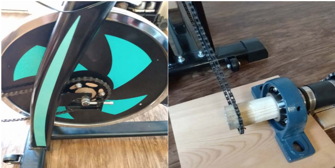
Figure 53. Stationary Bike with Mounted Gears and Chain
