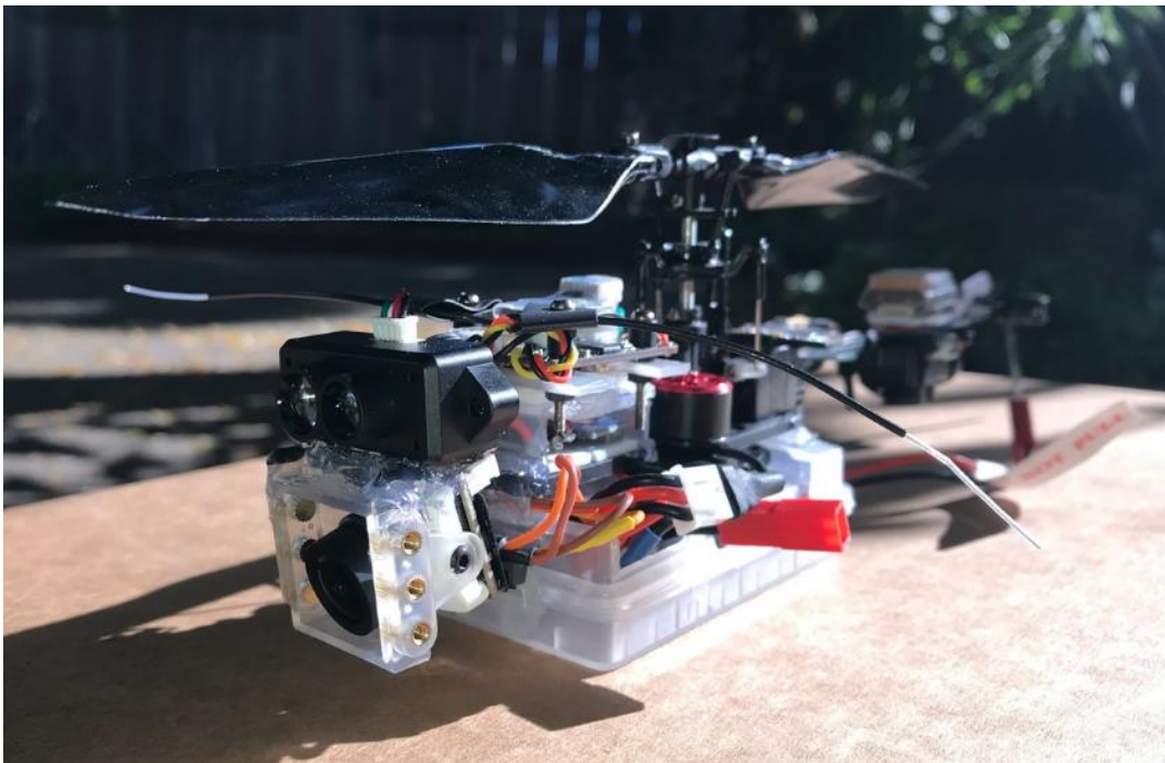
Figure 39. FRC COTS Drone Prototype (Front-Corner View).
