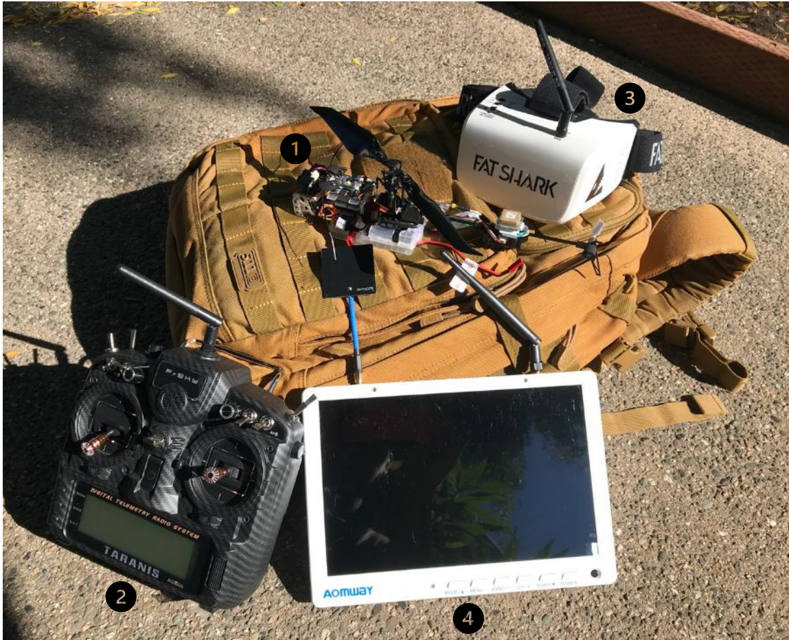
The four-part PRRD kit is composed of the (1) FRC COTS UAV, (2) FrSky Taranis X9D Plus SE 2019 handheld controller, (3) Fat Shark Recon V3 FPV Goggles, and (4) Aomway HD588 V2 HD FPV Monitor.
