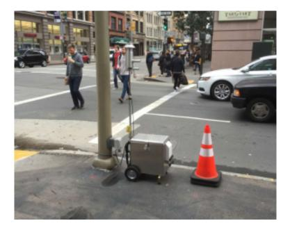
Figure 10.4 BioWatch Gen 2 Aerosol Collector (Mercer, 2016)
