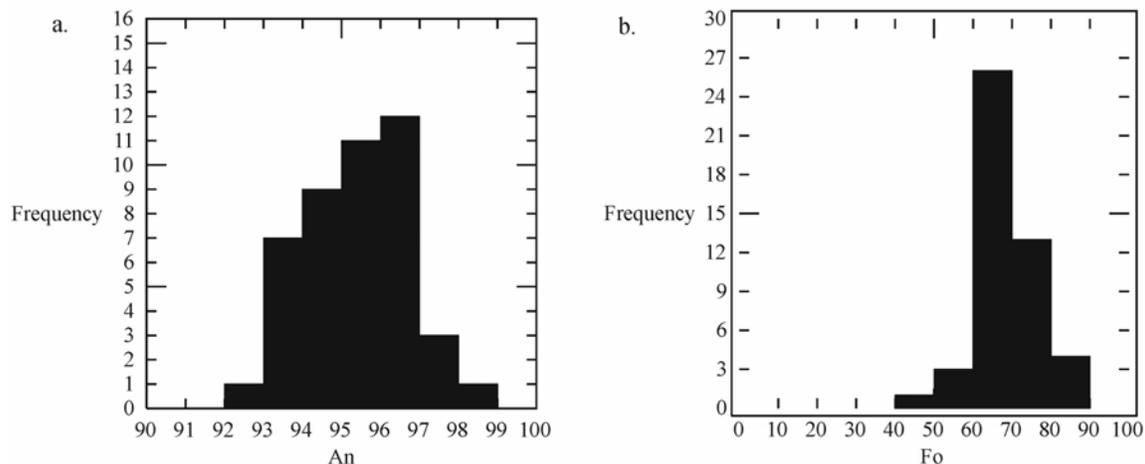
Fig. 8. Compositions of plagioclase and olivine in SaU 300. Boxes are for matrix minerals and mineral fragments. a) Anorthite content of plagioclase in SaU 300.  $N = 44$ ; mean = 95.3; std. dev. = 1.2. b) Forsterite content of olivine (atomic Mg/[Mg + Fe])  $N = 47$ ; mean = 67.4; std. dev. = 8.1.
