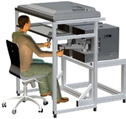
Figure 3.2A. Kinarm-the robotic equipment used to program and administer the motor learning task.
