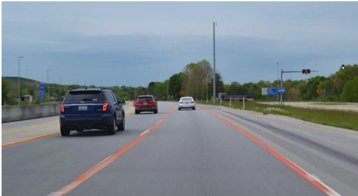
Figure 4.3 Waterborne Orange Paint After 250 Days
