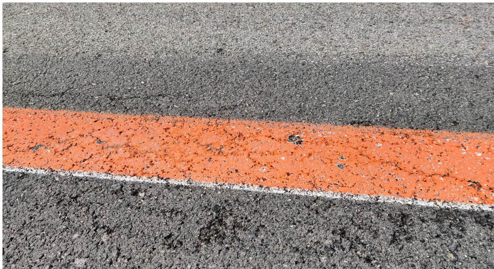
Figure 4.2 Waterborne Orange Paint After 100 Days
