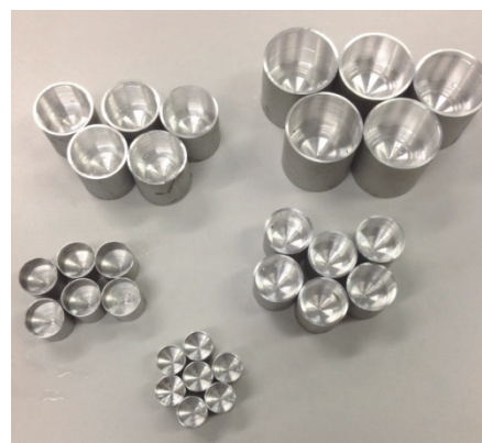
Fig. 2. Five sets of scale containers.
