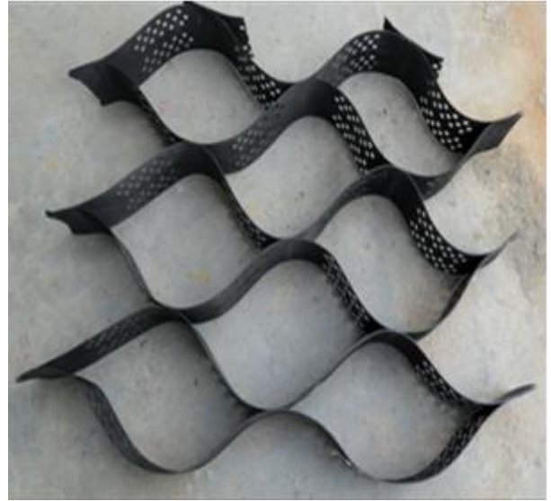
Figure 2. Typical geocell used in the study
