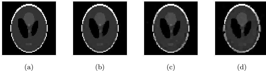
Fig. 3: Reconstruction of CT image using Total-Variation Augmented Lagrangian Method with measurement matrix of 4 different sizes: (a) 4096 \times 4096 (b) 2048 \times 4096 (c) 1365 \times 4096 (d) 1024 \times 4096 .
