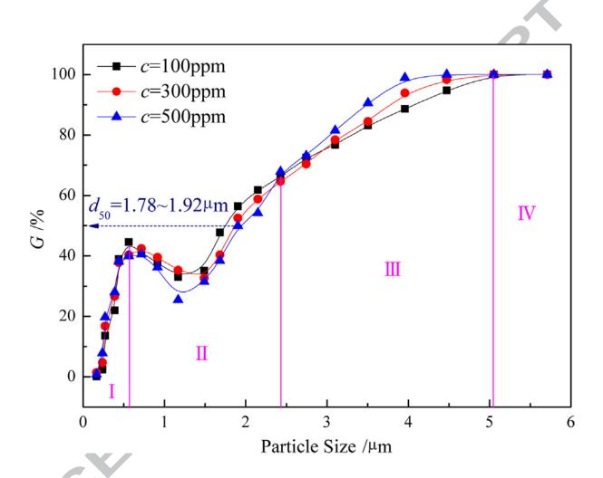
Figure 1 Actual efficiency curves reported by Lv et al. [2]. Similarity with the curve reported by Majumder et al. [2] (Figure 2) may be noted. Both report near zero efficiency of near zero sized particles, followed by an increase in efficiency. This is followed by a decrease in efficiency till it reaches a minimum and then a monotonic increase with size..
