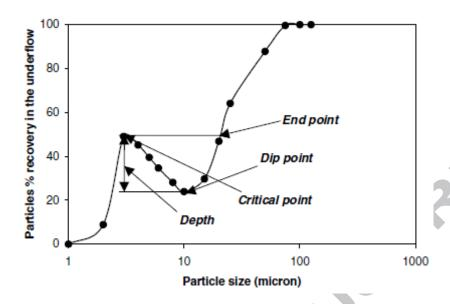
Figure 2. Efficiency curve showing a fish hook as reported by Majumder et al. [7]. The shape of this curve is distinctly different from all other efficiency curves reporting fish hook. None of them show the initial increase with size till 'critical point'.
