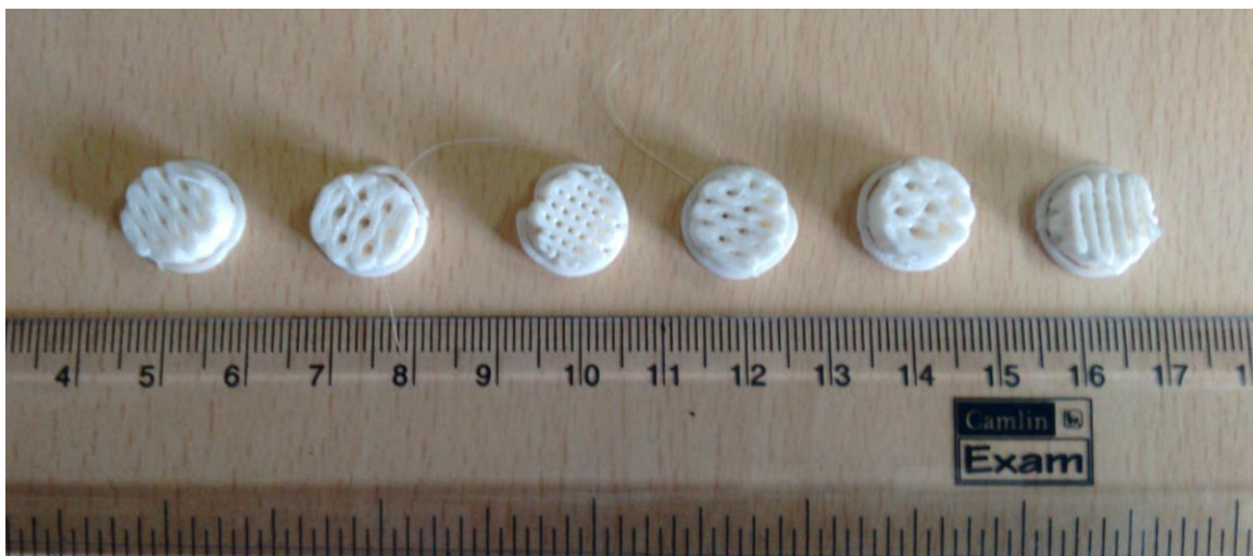
Figure – 5.5: Scaffolds for cell culture 16mm diameter honeycomb & rectilinear pattern
