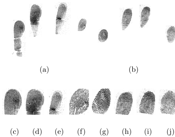
Fig. 4.4: Illustration of sequence of steps of de-noising slap fingerprints for accurate slap fingerprint segmentation: (a) noise-free slap of high noise, (b) noise-free slap of low noise, (c,d,e,f) are segmented fingers of noise-free slap of high noise, and (g,h,i,j) are segmented fingers of noise-free slap of low noise.
