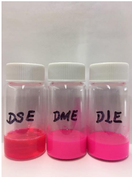
Figure 3.5 Photos of DiI-loaded NEs. DiI loaded SE (DSE, 0.2 mg/mL) had a transparent appearance whilst DiI loaded ME (DME, 1 mg/mL) and LE (DLE, 1 mg/mL) were milky.
