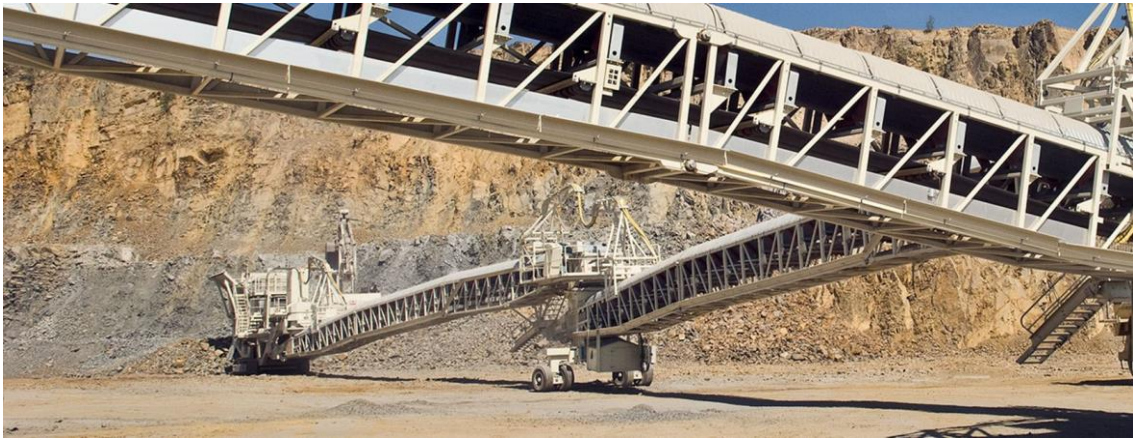
Figure 2-7. A portable conveyor belt in a limestone mine (Metso) [51]
