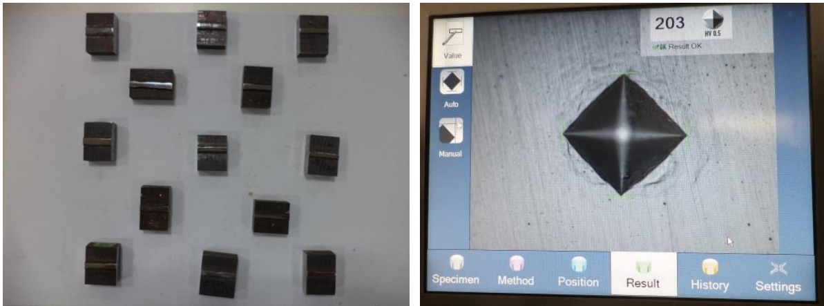
Figure 8: (a) A polished weld bead samples (b) diamond indent display of diagonal and hardness values
