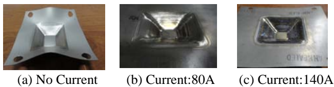
Fig 7: Pictures of formed components at no current, 80 amperes current and 140amperes current
