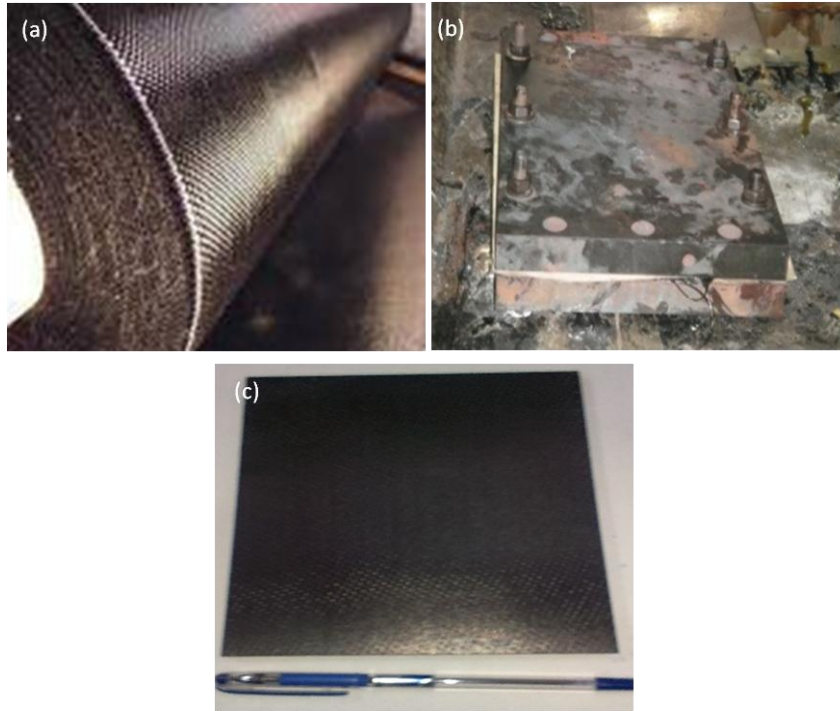
Figure.5.2. (a) Carbon fabric roll from which fabric layers of required dimensions were collected (b) Die plates used to sandwich the stacked fabric layers (c) A_f -CNF- C-epoxy composite fabricated for mechanical property evaluation.
