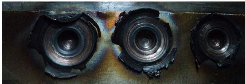
Figure 16: Photograph showing Optimization of Plunge depth for AISI-316L
