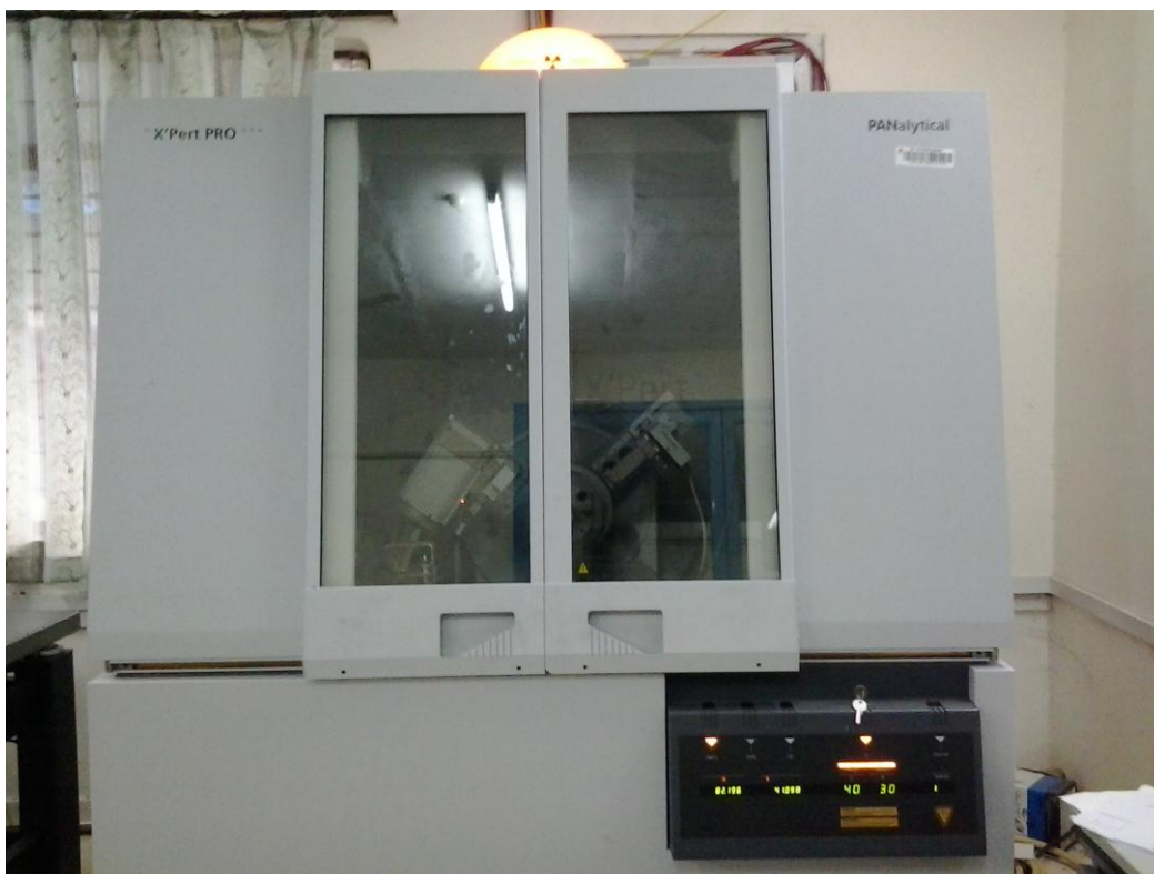
Fig 3.2.2.1: The laboratory instrument used X-ray diffraction studies for structural analysis.
