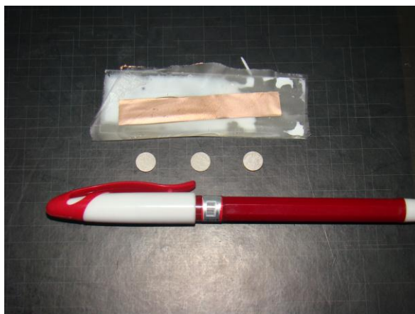
Figure 3.6 Picture of the synthesized and electroded NBT ceramic pellets and PVDF thick film
