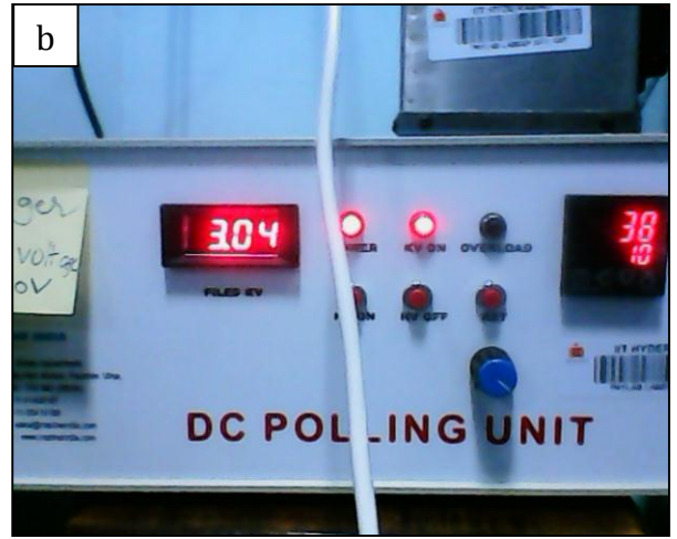
Fig. 3.7: Setup for poling a) Electrodes, Crucible, Heater b) DC field supply monitoring unit.
