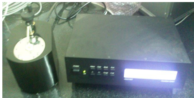
Fig.3.12 Piezometer system setup for d_{33} measurement
