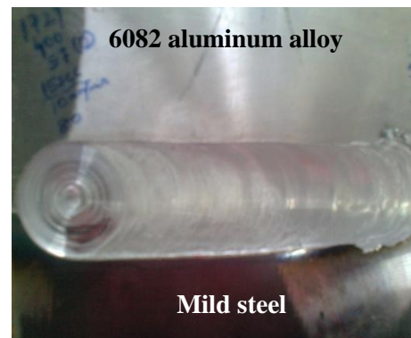
Figure. 4. Friction stir butt welded sample of Al 6082 alloy (white colour) and Mild steel (black colour)
