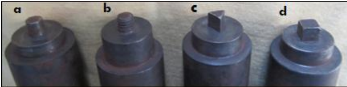
Figure 4.1: different pin profiles; (a) Straight cylindrical. (b) Threaded. (c) Triangular (d) Square
