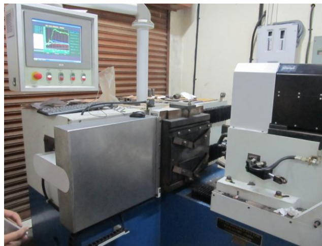
Figure 3.5: Friction Stir Welding (FSW) Machine
