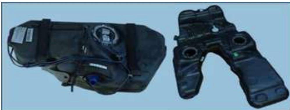
Figure1.1 : Single chamber tank (left) and saddle tank (Right) [13]
