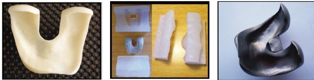
a) Femoral model using FDM b) Silicon mould c) Fabricated by casting
