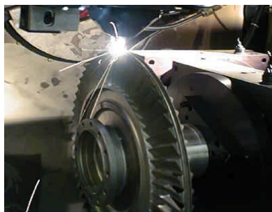
(c) LENS used for refurbishing a turbine
