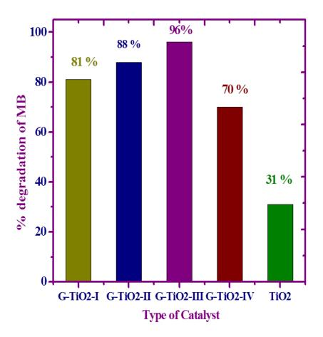
Percentage degradation of methylene blue dye with all combustion synthesized catalysts upon exposure to direct sunlight in 60 min. C0 = 10 mg/l, Catalyst amount =1gm/l.
