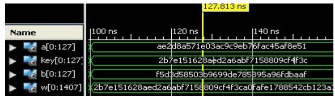
Figure 7: Output Waveform for Encryption with the input plaintext, key, ciphertext and the expanded key shown.
