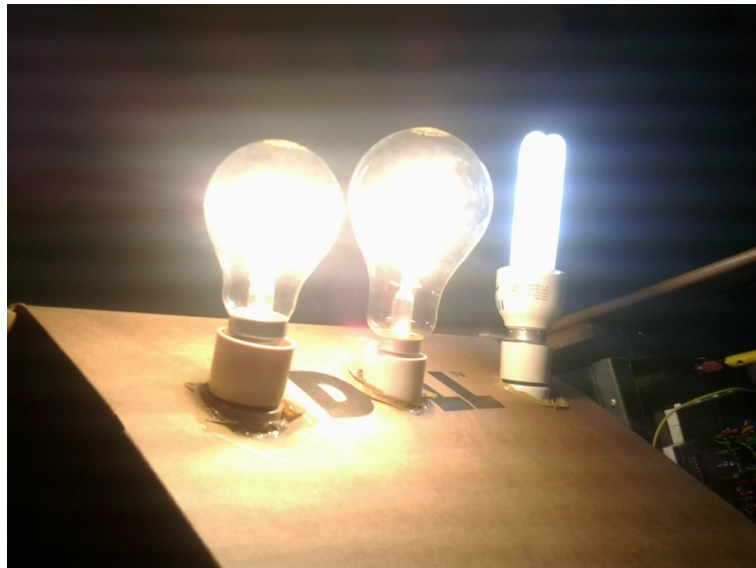
Figure 5.7: Three random loads of which two are monitored loads and one is the load stealing power
