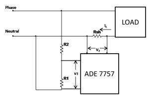
Fig 3. The basic block diagram showing the voltage and current inputs to the metering IC ADE7757
