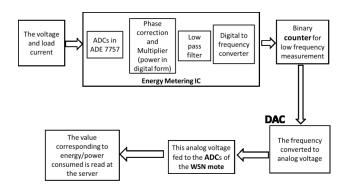
Fig 2. Basic block diagram of the system developed
