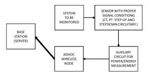
Fig1. System architecture for the power monitoring system
