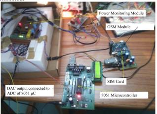
Fig.4. The implementation with the GSM module.
