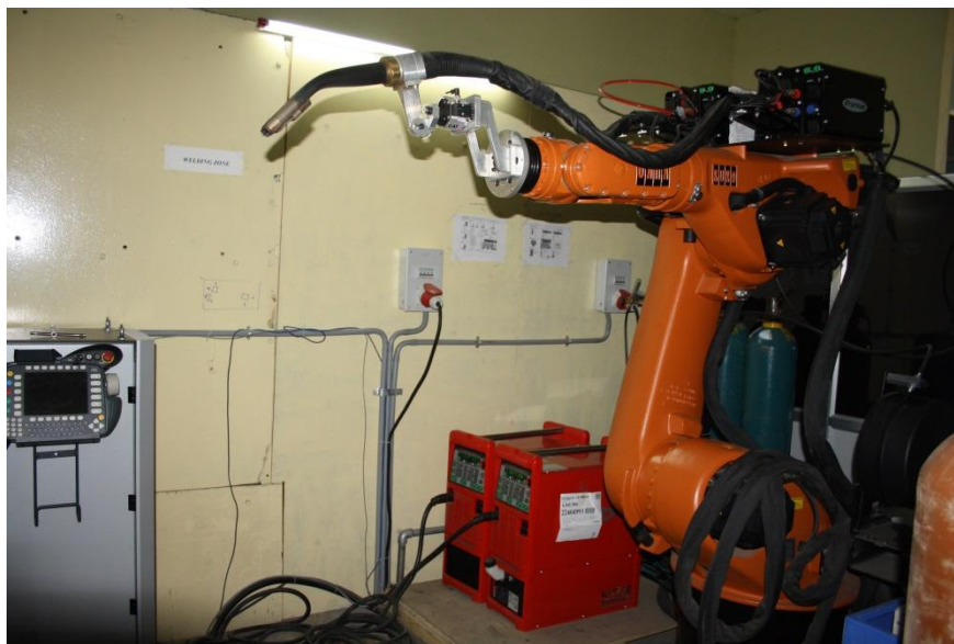
Figure 4.2: Welding deposition system integrated with Robot machine
