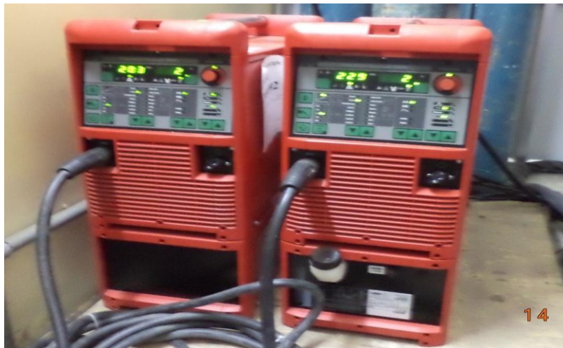
Figure 4.3: Complete welding system based on the power source Time Twin Digital 5000
