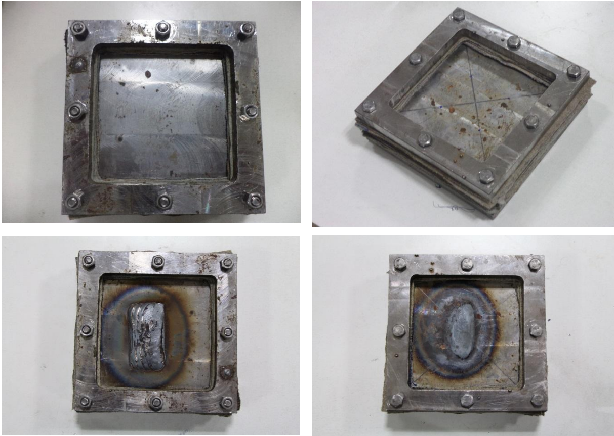
Figure 4.5: Different orientation of fixtures before and after the deposition
