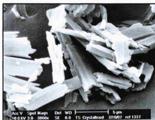
Figure 2.4.1.1: TS crystallised from absolute ethanol without retardant.
