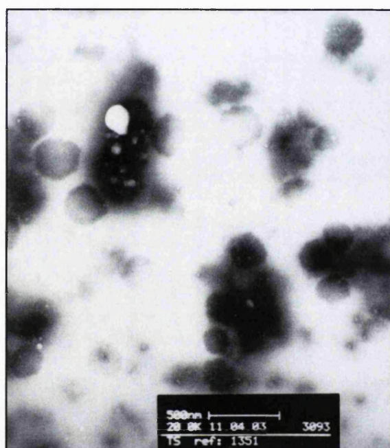
Figure 4.4.4.3: TEM image of TS nanoparticles, evidence of spherical structure present.
