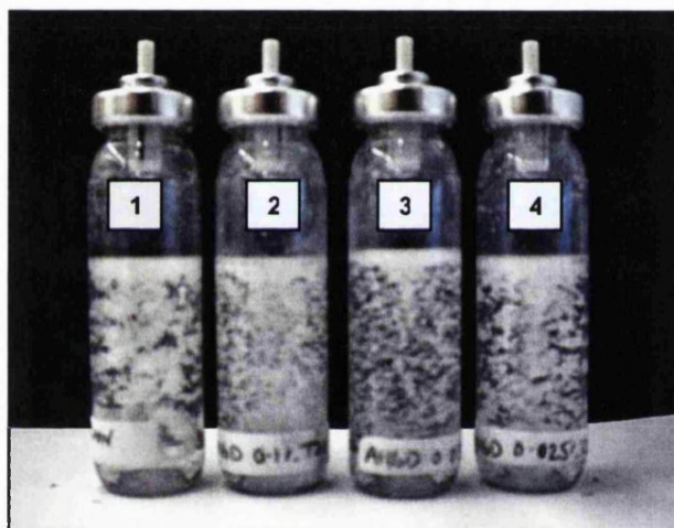
Figure 6.4.1.1: Flocculation in HFA formulations of SR-TS microparticles (10.0 mg): 1 = surfactant free, 2 = 0.1% w/v Tween 20, 3 = 0.05% w/v Tween 20, 4 = 0.025% w/v Tween 20. Photograph taken 10 sec following vigorous shaking (10 sec). Other surfactants displayed identical behaviour.
