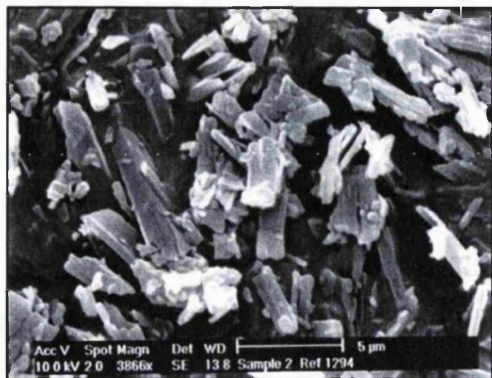
Figure 2.4.5.4: TS crystallized from 2% w/v L64/2% w/v L101 in absolute ethanol.
