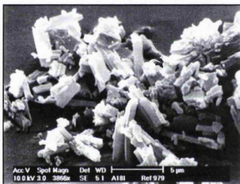
Figure 2.4.5.1: TS crystallized from 4% L44 w/v in absolute ethanol.
