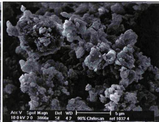
Figure 3.4.3.2: SEM image of 10:90 TS:CS microparticles (milled product).
