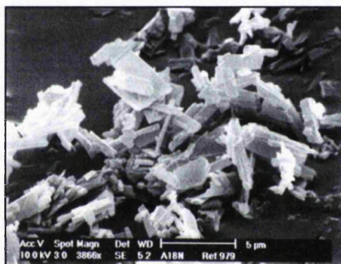
Figure 2.4.5.2: TS crystallized from 10% w/v L64 in absolute ethanol.
