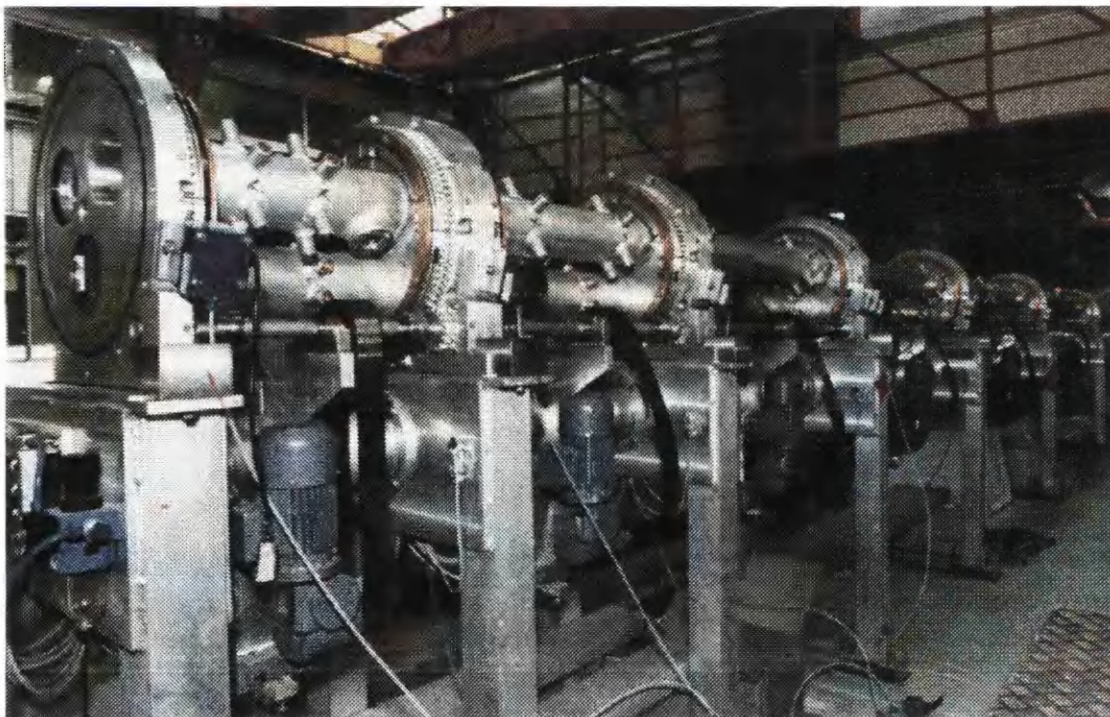
Figure 2.14: Picture of the primary collimation system on D22. (Taken from the ILL World Wide Web Site http://www.ill.fr ).
