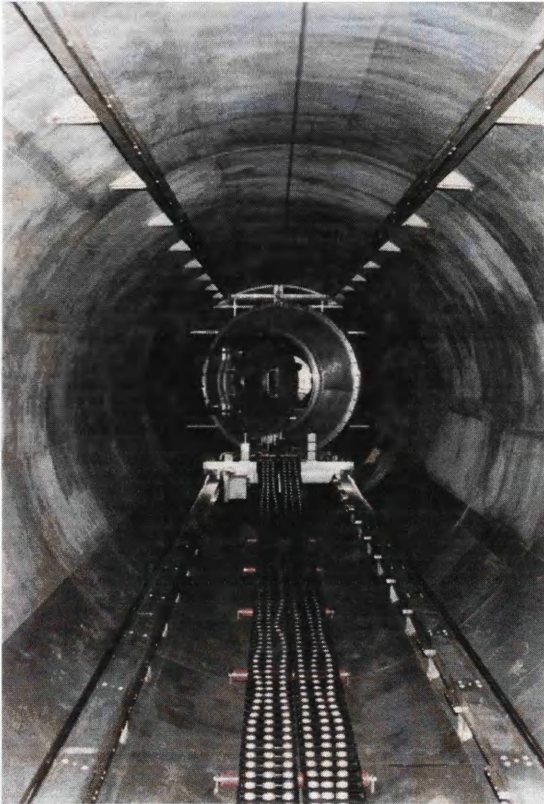
Figure 2.19: D22 multidetector housing inside the vacuum tube. (Taken from the ILL World Wide Web Site http://www.ill.fr ).
