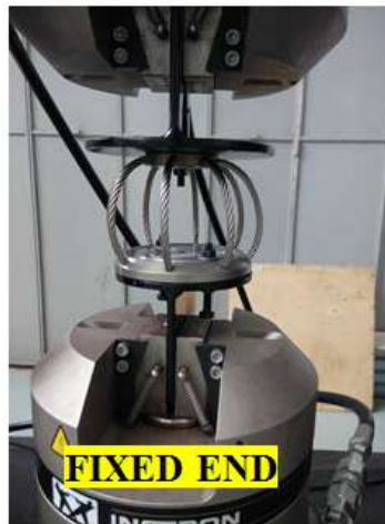
Figure 4. Loading Test of WRI in Vertical Directions
