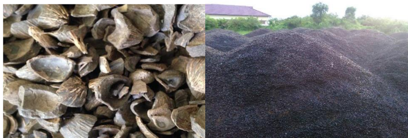
Figure 1. (a) Oil palm shell (OPS) (b) Oil palm shell solid waste in oil palm factory.
