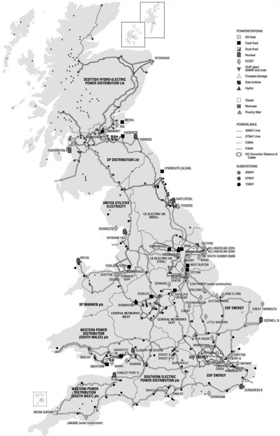
Figure 6: Great Britain Electricity Network
