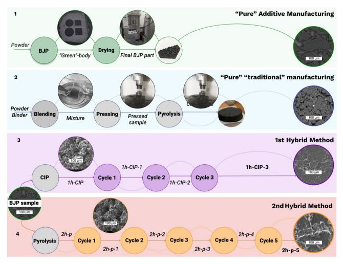
**Figure 2.** Process flow showing production of graphite using different production routes where *BJP* Binder Jetting Printing, *CM* compacted moulding, *CIP* Cold Isostatic Pressing, Cycle is the sequence of Impregnation—Drying—Pyrolysis.
