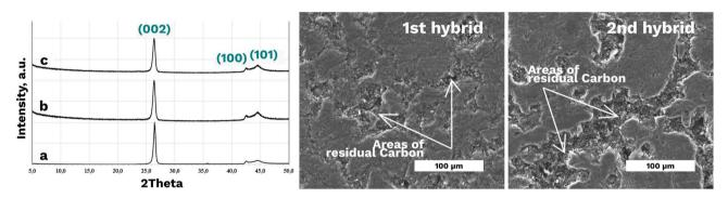
**Figure 7.** XRD spectra of the: (**a**') BJP; (**a**") 2 h-p-5 sample; (**a**<sup>"''</sup>) 1 h-CIP-3 sample; (**b**,**c**) SEM images of the 1st hybrid sample (1 h-CIP-3) and 2nd hybrid sample (2 h-p-5).
