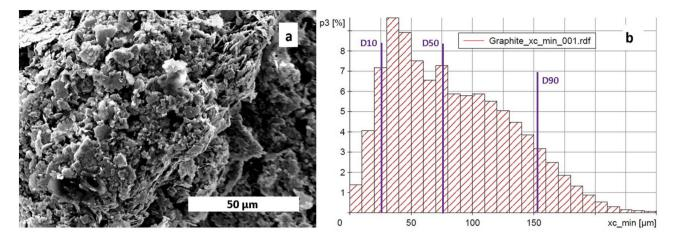
Figure 3. (a) Scanning electron microscopy (SEM) image showing graphite powder morphology and (b) Particle size distribution of the graphite powder used.
