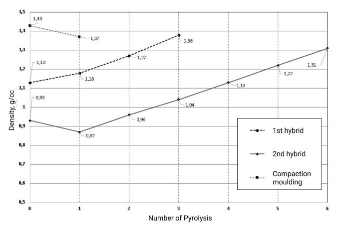
**Figure 5.** Dependence of the hybrid and compacted samples density on the number of pyrolysis cycles. 2nd to 6th pyrolysis was applied after PRBI. For compacted sample as initial density is the density before pyrolysis.
