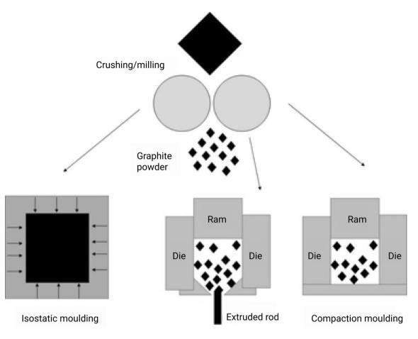
**Figure 1.** Production techniques for graphite structures (left) isostatic pressing or moulding (middle) extrusion and (right) uniaxial compaction.
