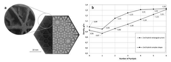
**Figure 9.** (a) Overview of graphite BJP complex structures densified through PRBI and pyrolysis cycles; (b) dependence of the hybrid complex-shape sample's density on the number of pyrolysis. The 2nd up to 6th pyrolysis was applied after PRBI.
