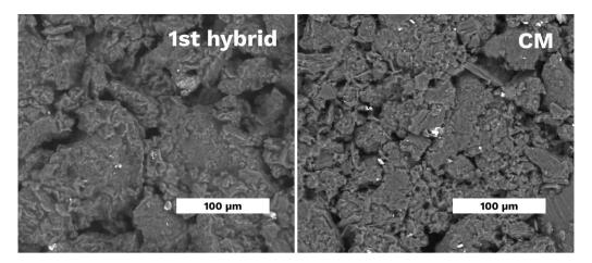
Figure 6. SEM images of the 1st hybrid sample (1 h-CIP-5) and CM compaction moulded sample.
