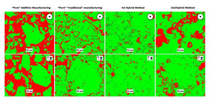
**Figure 4.** Image analysis of optical microscopy images of crosscuts in XY- and Z-planes. The black arrow points at the build/pressing direction (Z), i.e., perpendicular to the layers; the black circle with the point in the center corresponds to XY plane–parallel to layers.
