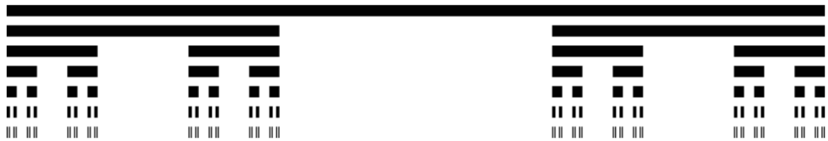
Figure 5. The Cantor Set with a Fractal Dimension of 0.6309.
