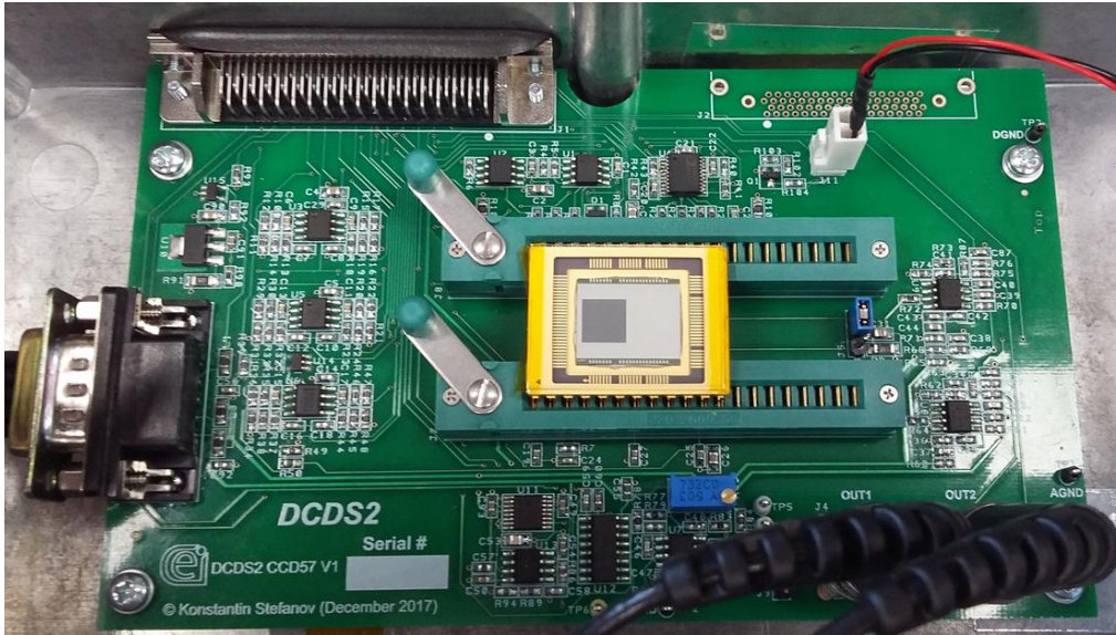
Figure 6-30: Photograph of the CCD57 mounted on the PCB with connectors to external power sources and data transmission lines.
