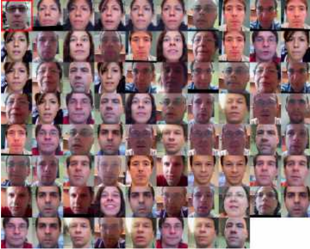
Figure 8. Master face (bordered in red) and all matching enrolled faces sorted from nearest to furthest for eval set of MOBIO database [21].
